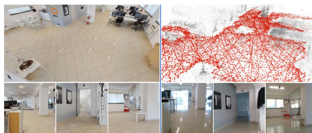
Fig. 2 On the left, a view of the geometrically accurate 3D model of the considered office environment. It allows the sampling of images from any position but it is limited in terms of photo-realism. On the right, a view of the 3D models of the same indoor environment, reconstructed following a Structure from Motion (SfM) (Schönberger & Frahm, 2016) pipeline. It contains a sparser collection of real-world images paired with their camera poses (each red marker represents the position of an image in the 3D model)
